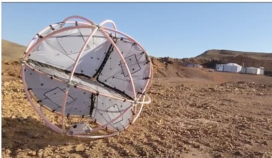
Figure 1: The Tumbleweed V3 Prototype rolling across the Negev desert, during the AMADEE20 Mars Analogous Mission [5].
