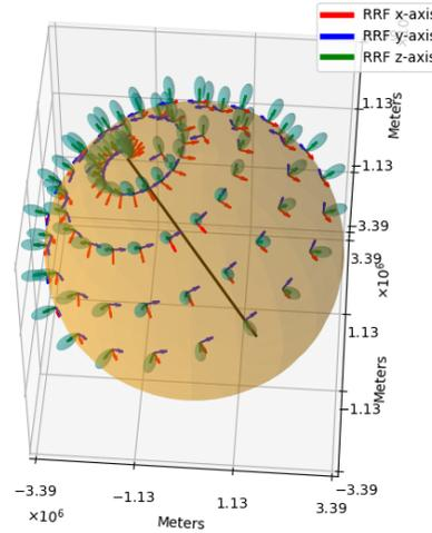
Fig. 3. Rover reference frames and the second antenna options (microstrip patch) radiation patterns for every 600th rover over 50k timesteps
