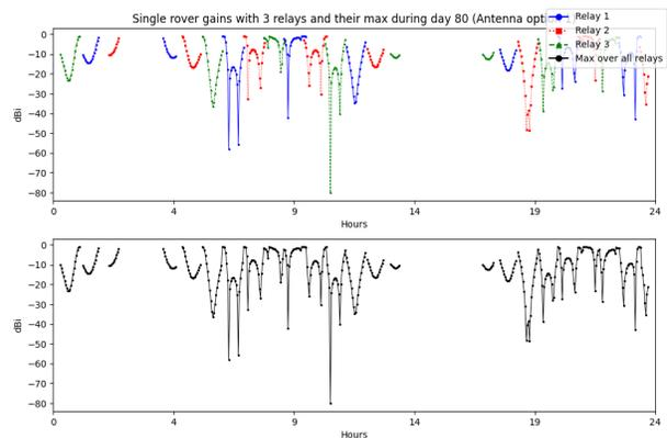
Fig. 8. The gains for a single rover with 3 relays (top), and the maximum gains over all relays (bottom) for the first antenna option during the 80th mission day
