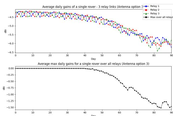
Fig. 13. The daily average gains for a rover and 3 relays (top) and their max over all relays (bottom) for antenna design option 3
