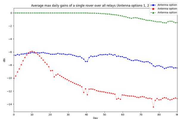
Fig. 14. Max gains of each antenna design over all three relays
