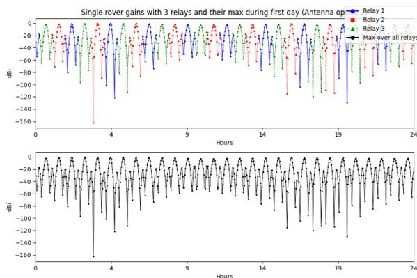
Fig. 6. The gains for a single rover with 3 relays (top), and the maximum gains over all relays (bottom) for the second antenna option during the first mission day
