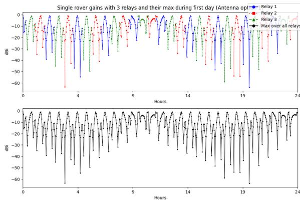
Fig. 5. The gains for a single rover with 3 relays (top), and the maximum gains over all relays (bottom) for the first antenna option during the first mission day
