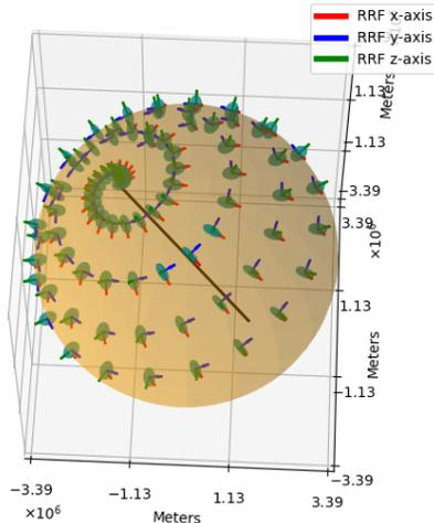
Fig. 2. Rover reference frames and the first antenna option (halfwave dipole) radiation patterns for every 600th rover over 50k timesteps
