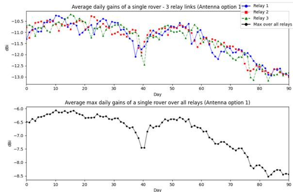
Fig. 11. The daily average gains for a rover and 3 relays (top) and their max over all relays (bottom) for antenna design option 1
