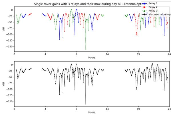
Fig. 9. The gains for a single rover with 3 relays (top), and the maximum gains over all relays (bottom) for the second antenna option during the 80th mission day
