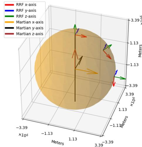
Fig. 1. Reference frames at three timesteps of a single rover travelling down on the xz-plane
