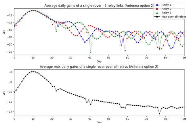
Fig. 12. The daily average gains for a rover and 3 relays (top) and their max over all relays (bottom) for antenna design option 2
