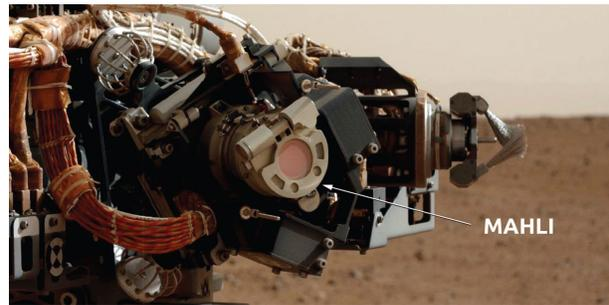
Figure 8: Mars Hand Lens Imager (MAHLI) attached to the Curiosity rover [46].
