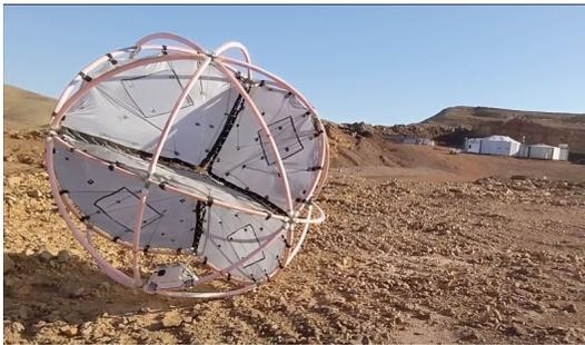
Figure 6: The Tumbleweed V3 Prototype rolling across the Negev desert, during the AMADEE20 Mars Analogous Mission[36].
