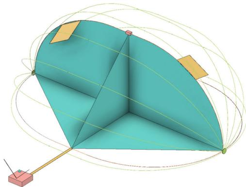
Figure 4: Simplified Tumbleweed Rover schematic in its stationary phase [29].
