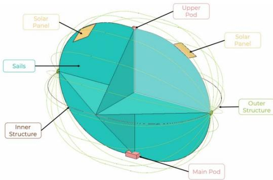
Figure 5: Simplified Tumbleweed Rover schematic [29].
