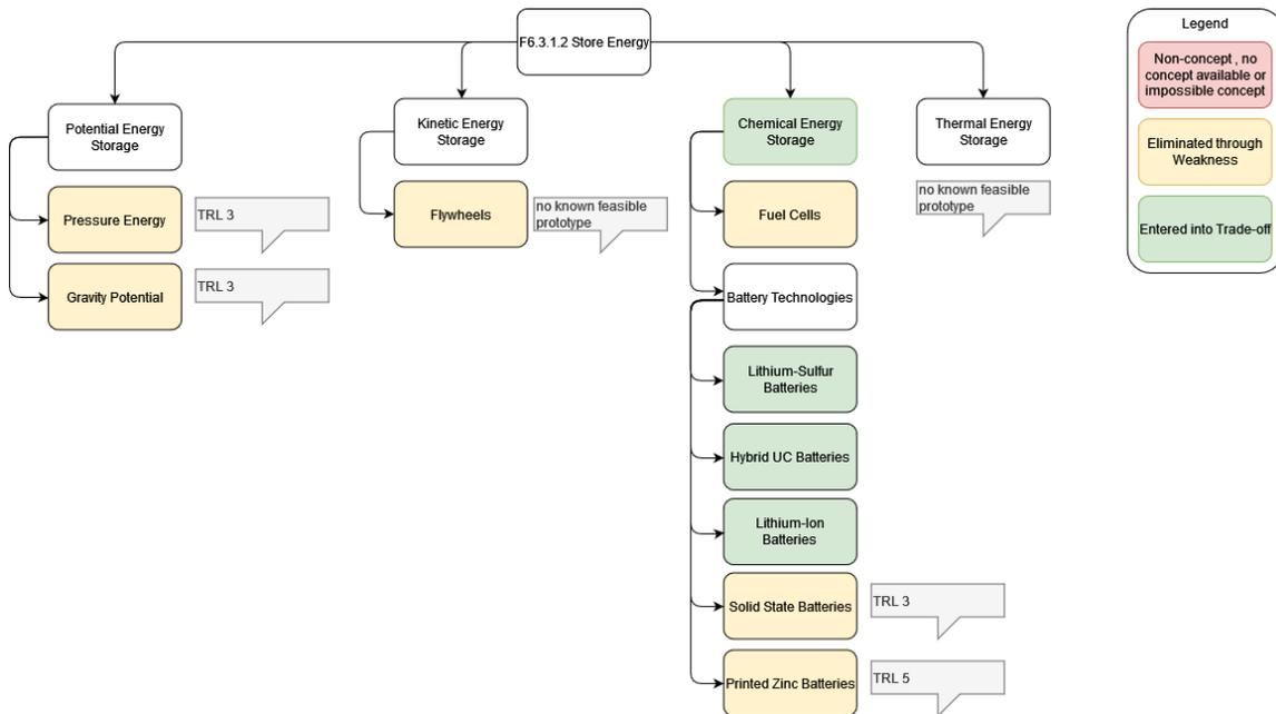
Figure 5.13: Design options/trade tree for the function F6.3.1.2 Store electrical energy.
