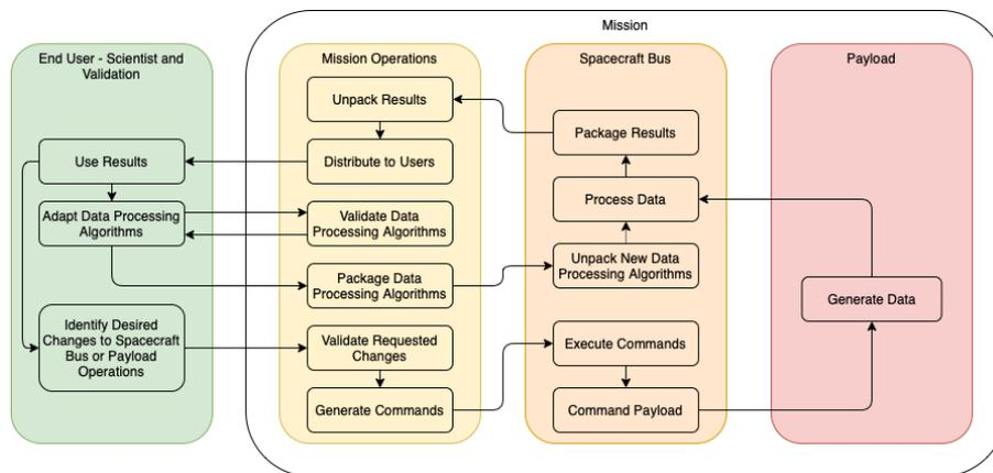
Figure 3.6: The user interaction diagram of the Tumbleweed Demonstrator Mission.
