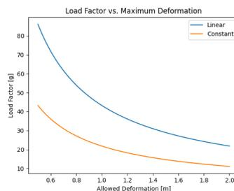
Figure 5.6: Worst- and best-case impact acceleration for pure drag-based landing at 4 km altitude
