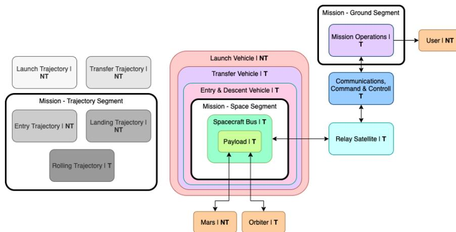
Figure 3.1: The logical architecture of the rover-only mission concept of the Tumbleweed Demonstrator Mission.
