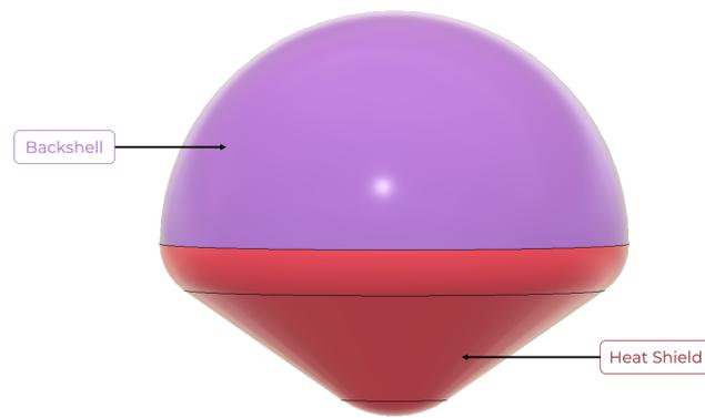
Figure 6.2: Conceptual design of the SCB concept with labelled subsystems
