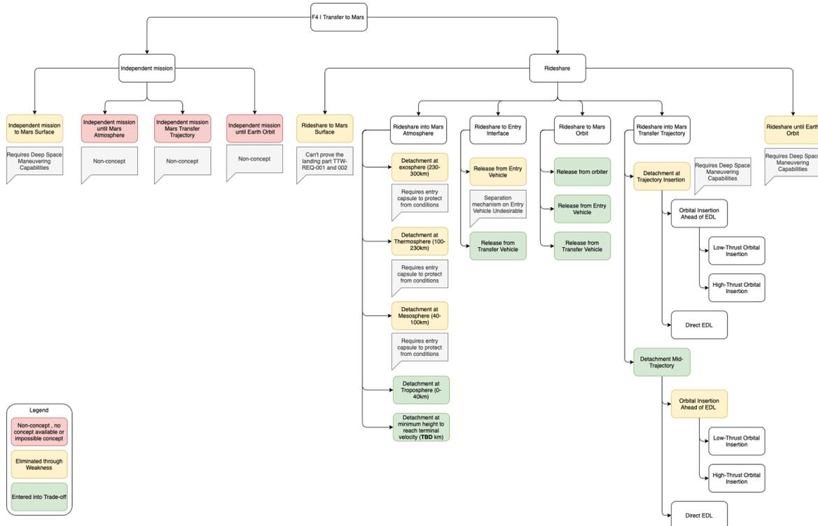
Figure 5.3: Design options/trade tree for the function F4 Transfer to Mars.
