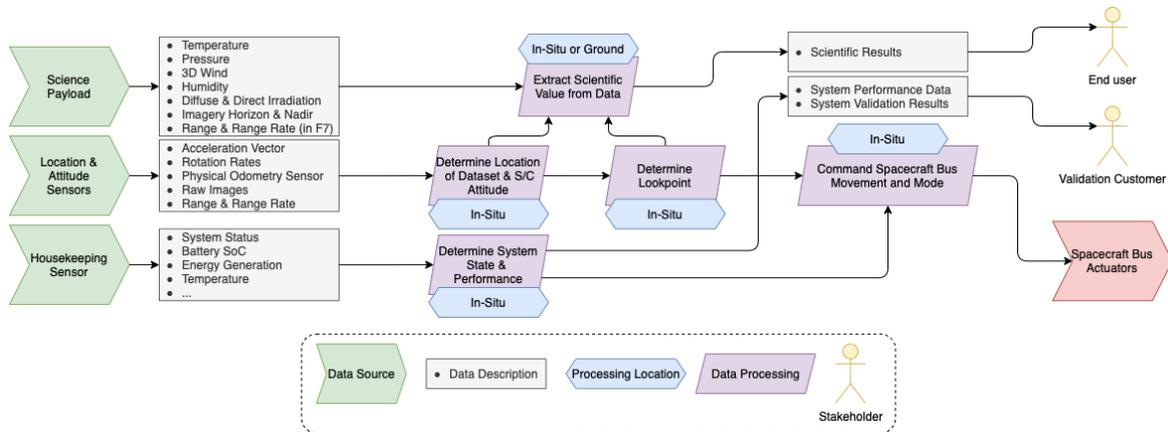
Figure 3.5: The data flow diagram of the Tumbleweed Demonstrator Mission.
