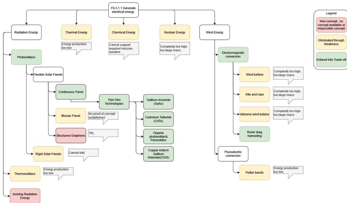
Figure 5.12: Design options/trade tree for the function F6.3.1.1 Generate electrical energy.
