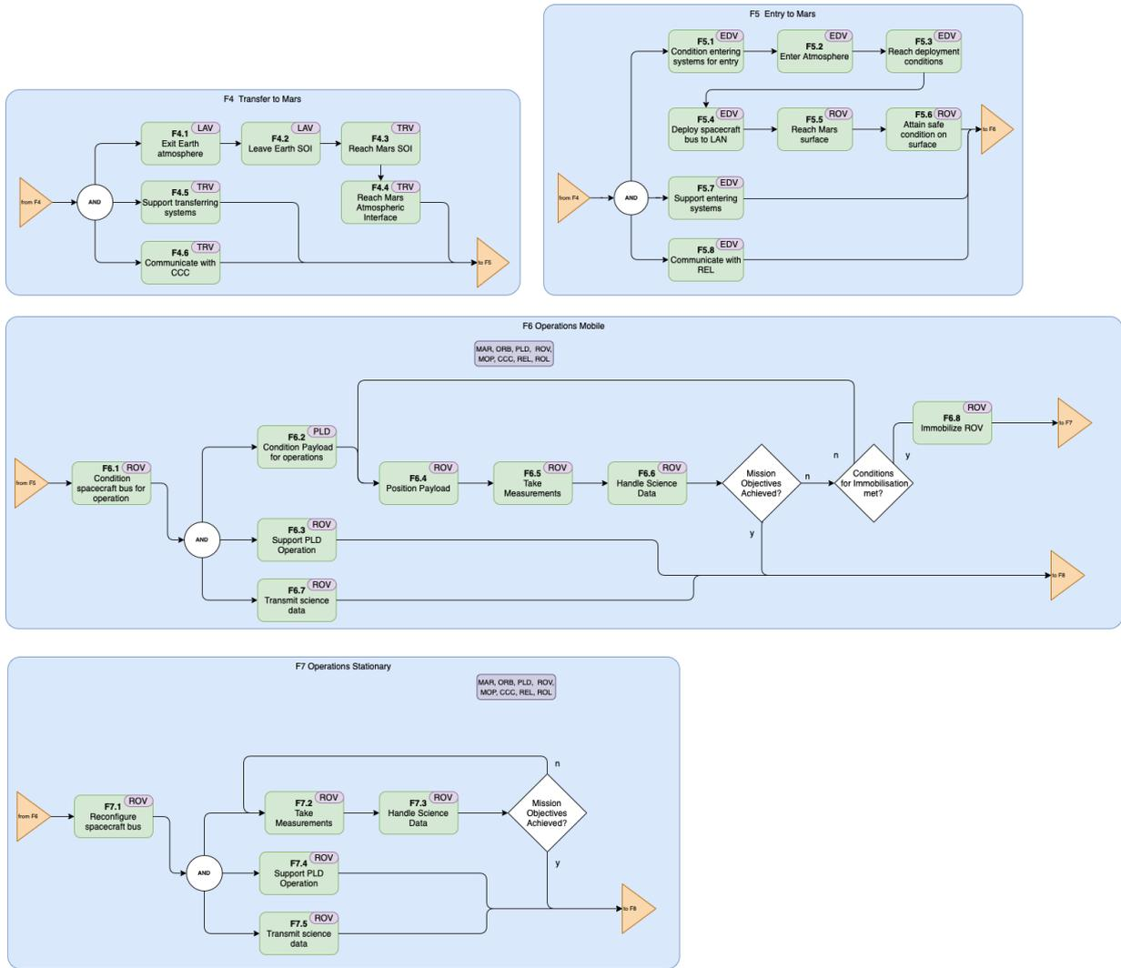
Figure 3.3: The second-level mission functions of the Tumbleweed Demonstrator Mission.
