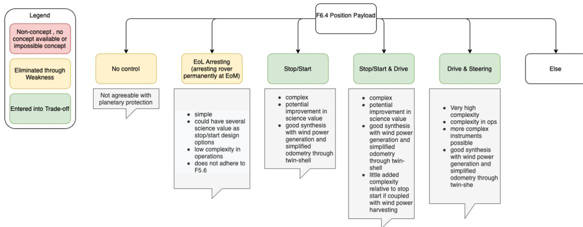
Figure 5.9: Design options/trade tree for the function F6.4 Rover Controllability.
