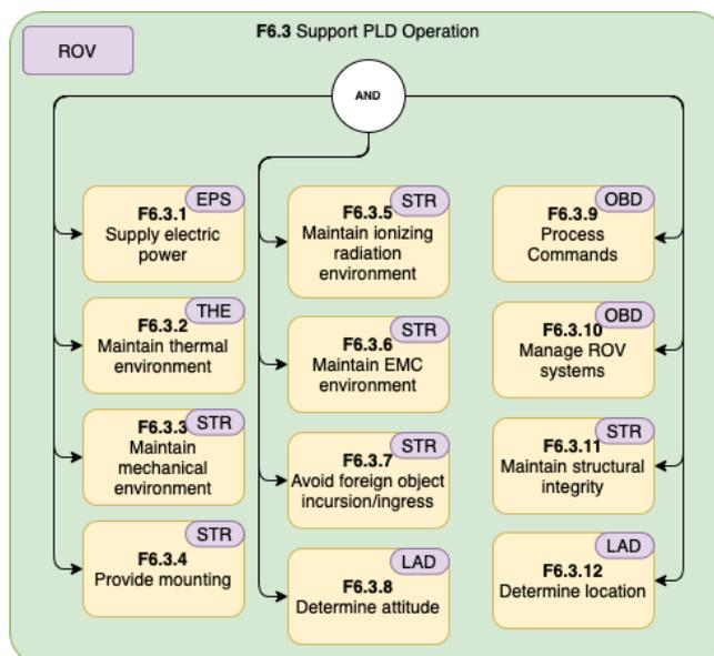
Figure 3.4: The third-level functions of function F6.3 of the Tumbleweed Demonstrator Mission.
