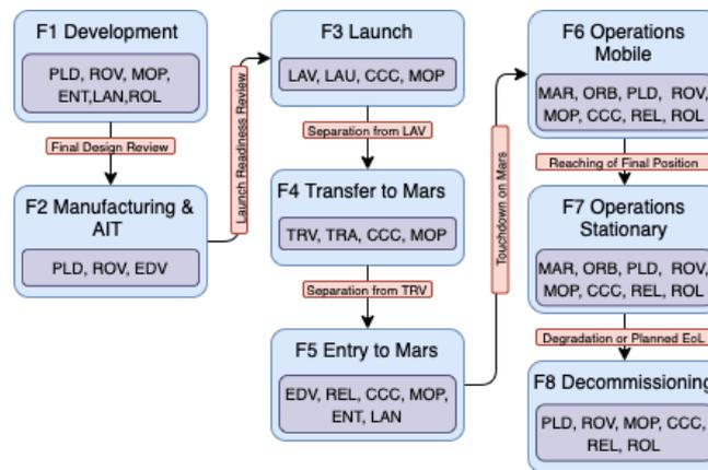
Figure 3.2: The mission phases of the Tumbleweed Demonstrator Mission.
