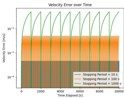
Figure 5.20: Theoretical velocity error over time
