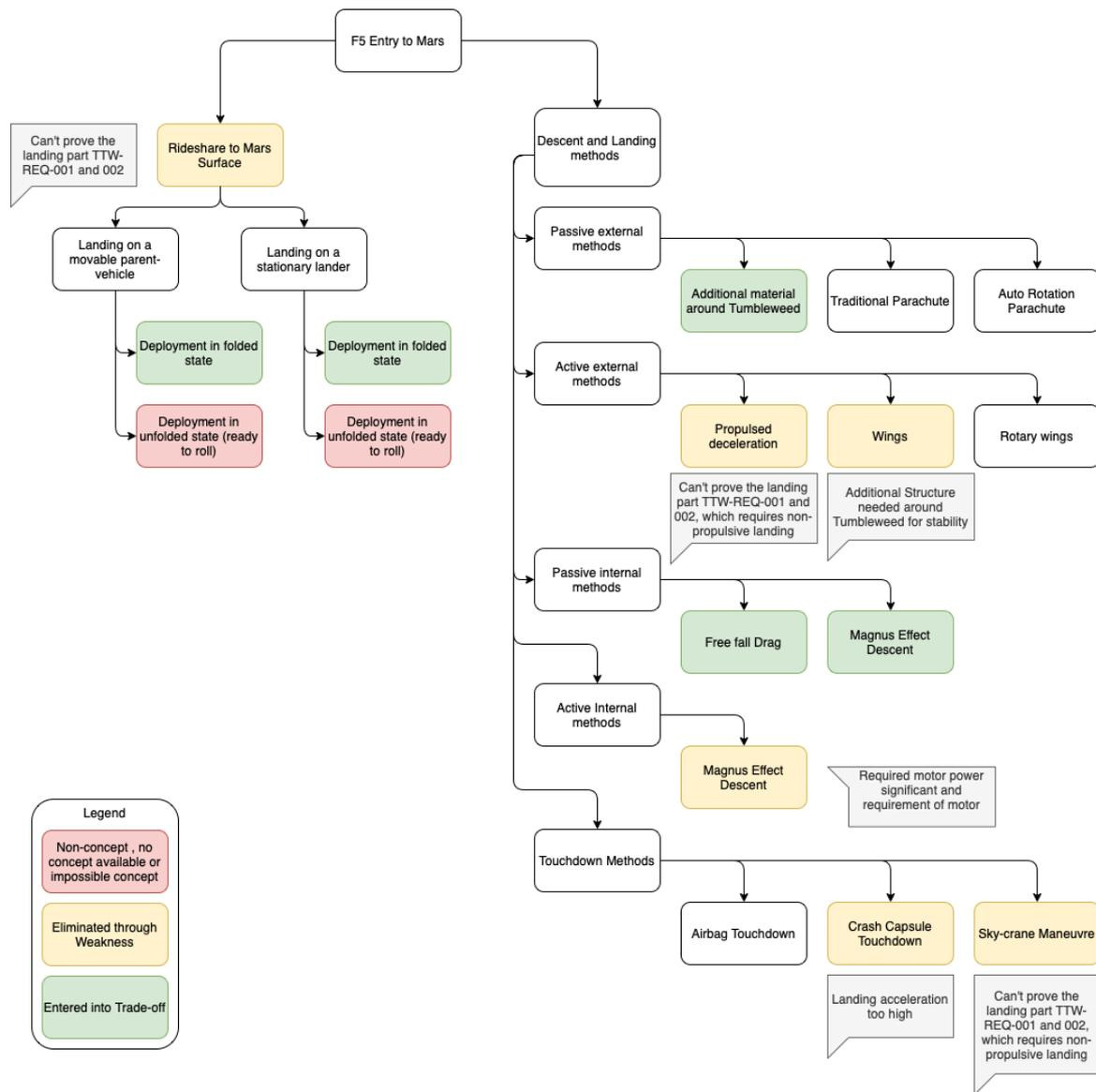
Figure 5.5: Design options/trade tree for the function F5.5 Reach Mars Surface.
