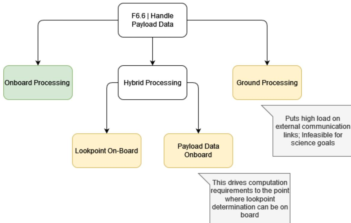
Figure 5.11: Design options/trade tree for the function F6.6 Handle Payload Data.
