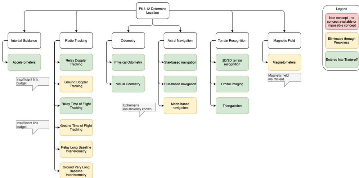
Figure 5.19: Design options/trade tree for the function F6.3.12 Location and Attitude Determination.
