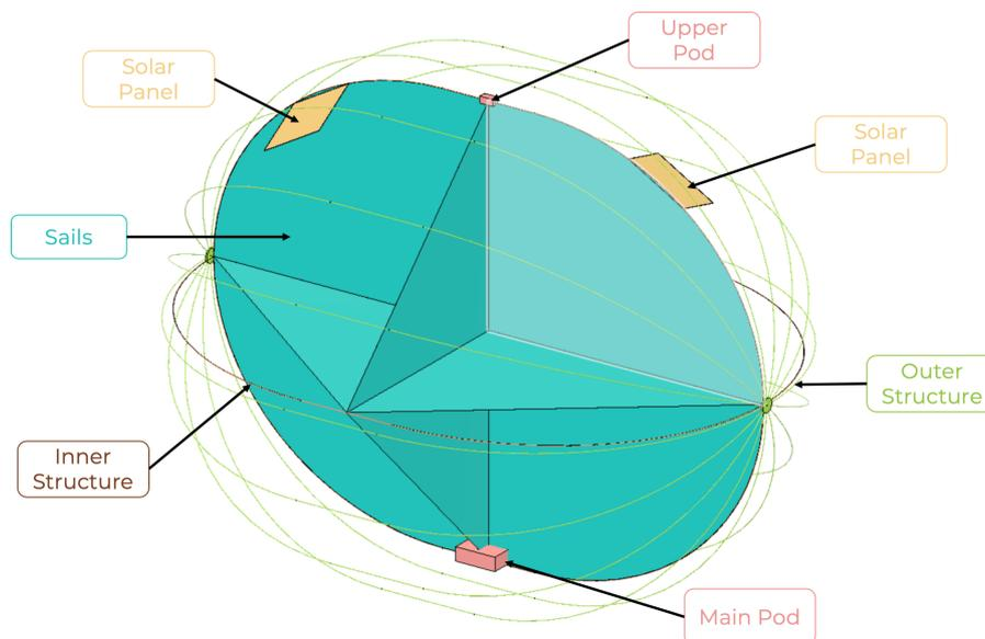
Figure 6.1: Conceptual design of the SCB concept with labelled subsystems
